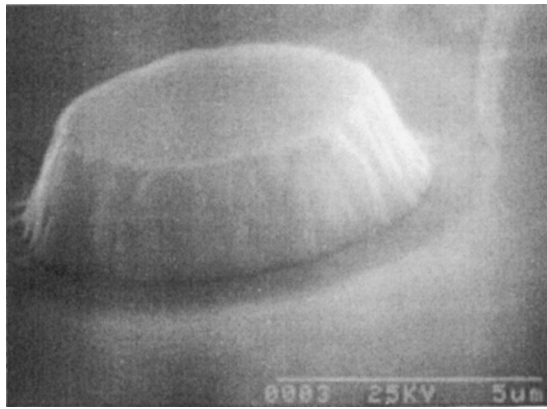
FIG. 1. SEM of an \text{In}_{0.22}\text{Ga}_{0.78}\text{N}/\text{In}_{0.06}\text{Ga}_{0.94}\text{N} MQW microdisk with a diameter of around 6.0\ \mu\text{m} .
